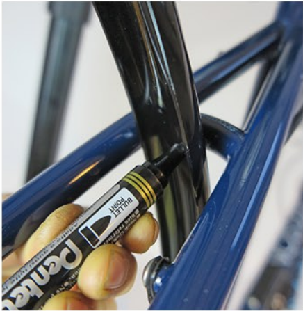
Mark up the rear fender for drilling point to secure to bridge.
