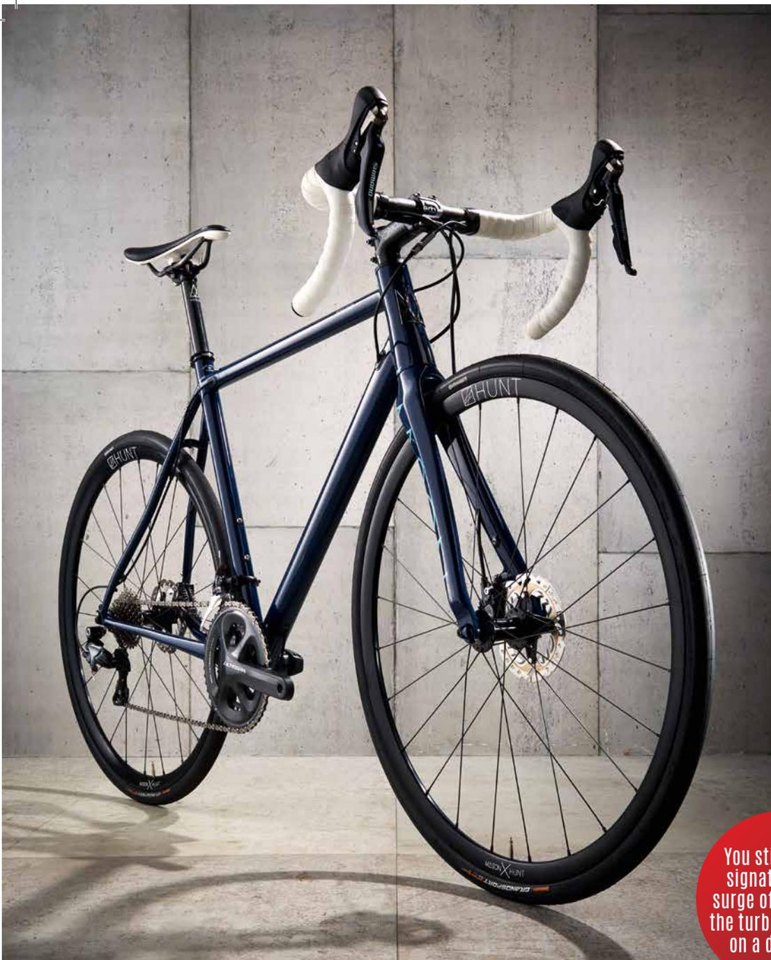
**+** **↓** Below Shimano disc brakes with 140mm rotors keep the Mason under control **Bottom** MultiPort inserts make for neat internal cable routing
