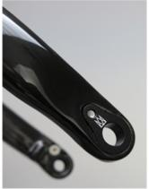
It is possible to remove the inserts and swap the sides if you would like your axle release lever on the drive-side or if the thread becomes damaged or worn through use.
