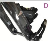
WARNING: It is important to remember that just a quarter turn of the release lever 'C' can be the difference between correct and incorrect closing force of the thru-axle lever. If thru-axle is not properly adjusted and the axle comes loose, the wheel may suddenly and unexpectedly eject from the fork. This may result in an accident causing personal injury or death.
