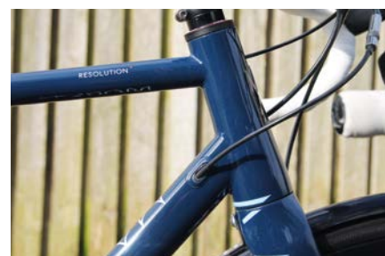
● (Above) The mudguard mounts on the Mason Resolution's carbon fork are well away from the disc calliper, so you don't need to bend the left-hand stay to fit (Below) Cables are routed internally, with different plug-in ports available for different setups, such as Di2
